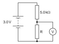
The reading on the voltmeter is 1.8 V.
